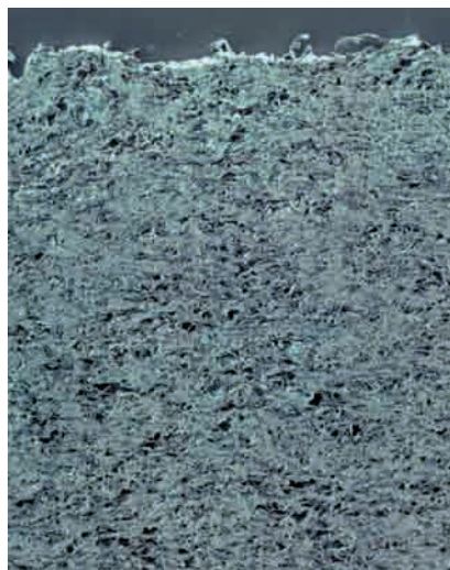
Depth filter sheet section under the microscope
